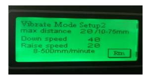
Enter the desired maximum distance or depth, down speed, and raise speed. With the example setup, the very bottom of a substrate will stay in solution for a total of 5 sec  $\times$  8 = 40 seconds, and the section 18 mm from the bottom will have a residence time of 5 seconds, and so on.
