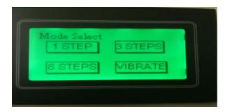
4. 1 STEP Mode is the simplest one but sufficient for most dip coating process. Press on "1 STEP", the following screen will show:
