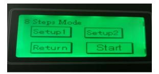
Press "Setup1" and enter total moving distance and three depths (in fact the speeds) that are desired, then press "Rtn" to go back to the "8 STEP" mode to continue the set up.
